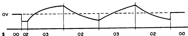
Fig. 2 Formation of search voltage through $02 and $03 (Pin 5 voltage)
